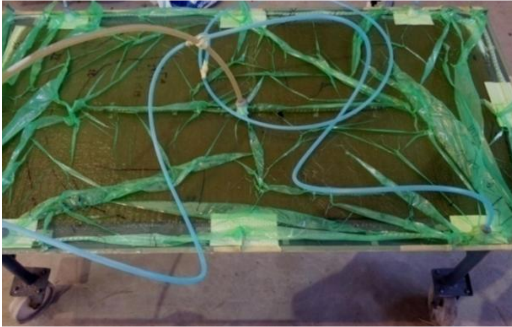
Fig.2. Preparation of fiberglass reinforced unsaturated polyester with infusion molding (VARTM).
