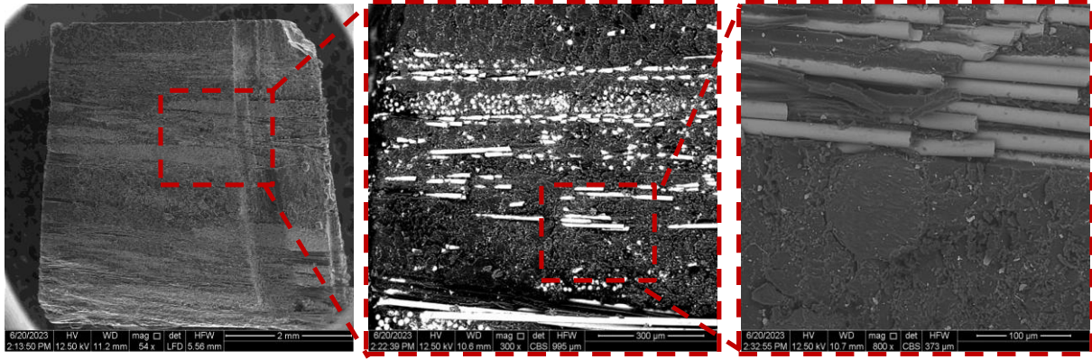
Fig.9. SEM micrograph of unsaturated polyester/glass composite before immersion.
