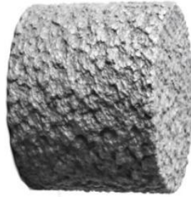
Fig.2. Surface Roughness Defects on a Cylindrical Test Specimen.
