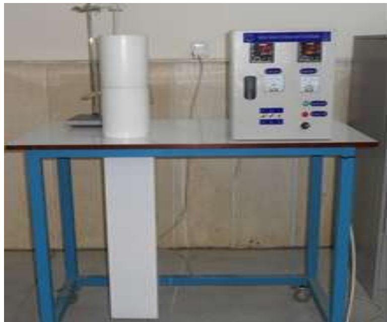
Fig.2. Thermal conductivity measurement apparatus
