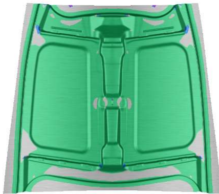
Fig.12. Formability of the rear door sash frame with a blank holder Force of 123.5T.
