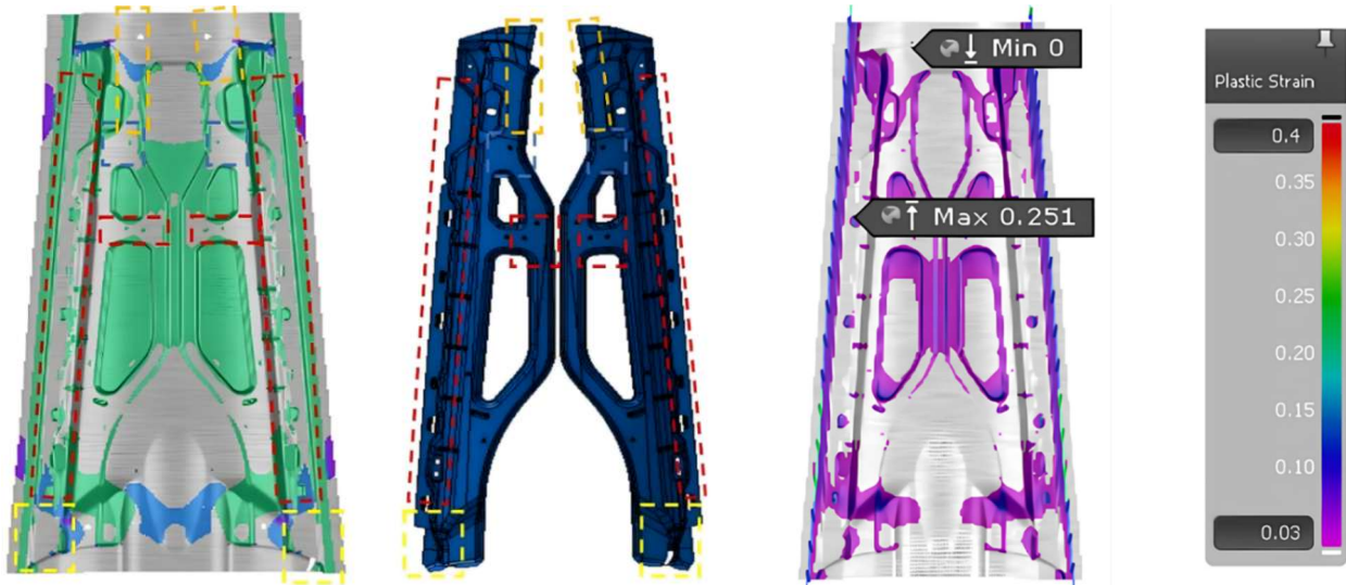
Fig.24. Formability of the sill outer reinforcement with a blank holder Force of 104T.
