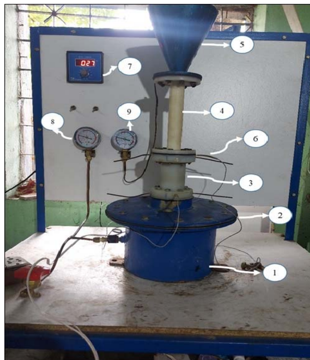
Fig.2. Experimental setup of thermoacoustic refrigerator.
