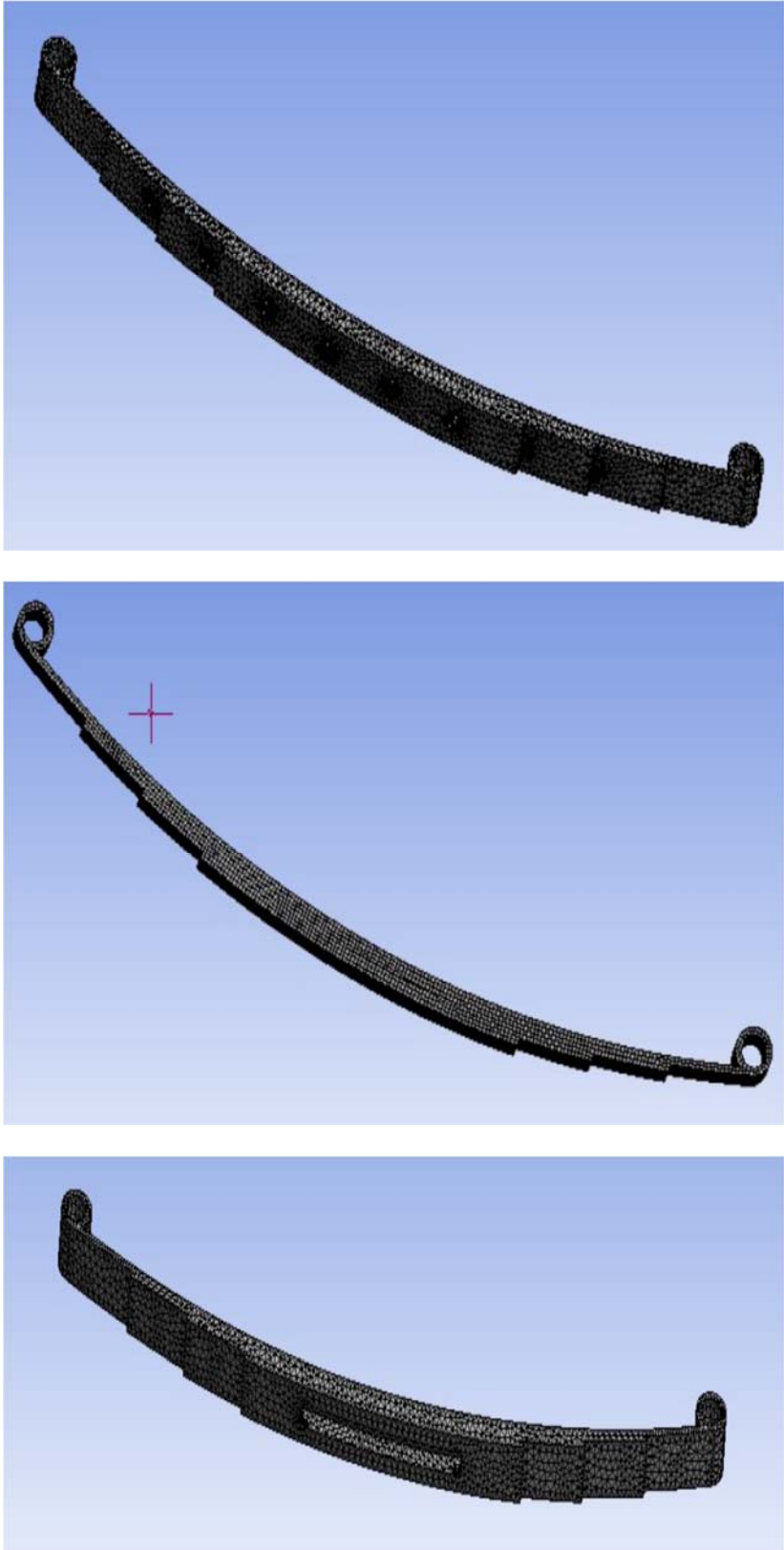
Fig.4. Fine meshing of traditional leaf spring assembly and the proposed designs.
