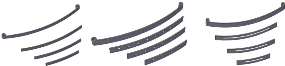
Fig.3. Unassembled view of leaf spring assembly.
