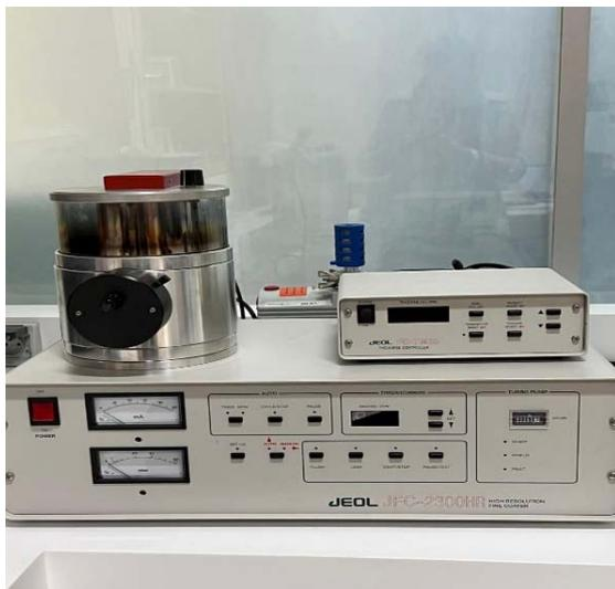
Fig.5. Sample preparation TI-6al-4v in JOEL-JFC.
