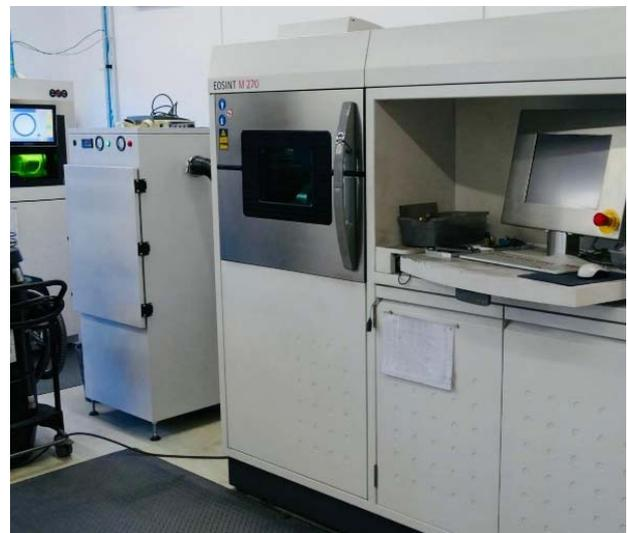
Fig.6. SLM machine EOSINT M270.
