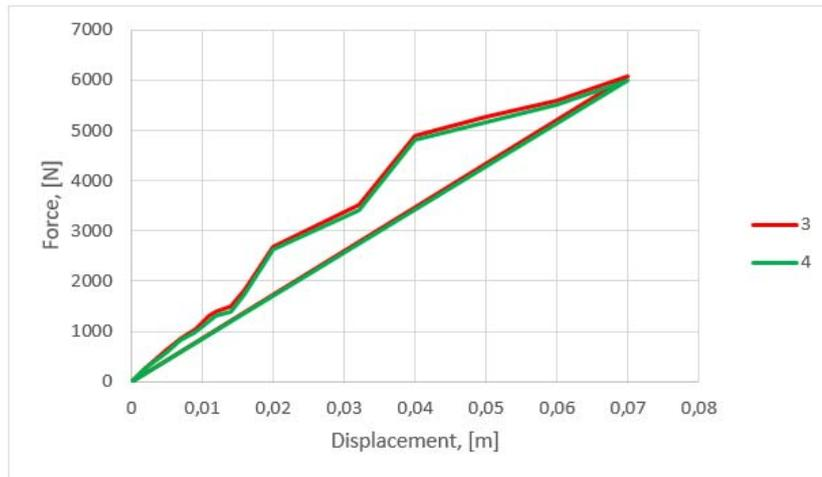
Fig.16. Modification of the deformation of a tire, size 205/55R16: 3 - tire depreciation; 4 - new tire.
