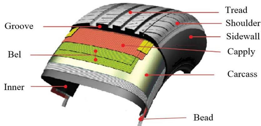
Fig.11. Structure of a radial car tire.
