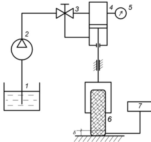
Fig.3. Measurement schematic diagram: 1 - reservoir; 2 - pump; 3 - regulator; 4 - cylinder; 5 - manometer; 6 - pneumatic tire; 7 - measuring device.
