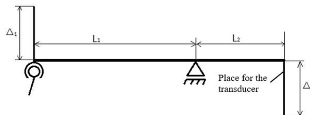
Fig.5. Lever system for measuring linear deformation,  $\Delta \text{ mm}$ .
