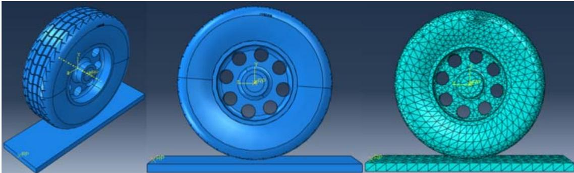
Fig.13. Three-dimensional FEM model of tire in Abaqus environment.
