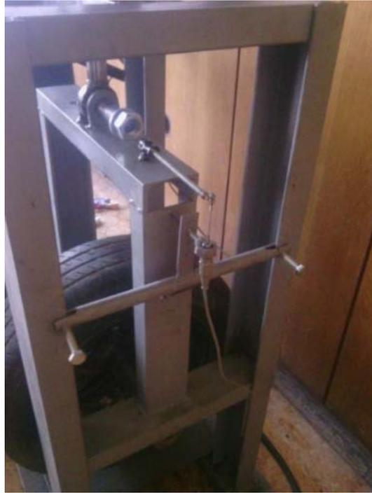
Fig.6. Photo of the lever system and the inductive converter mounted to it.
