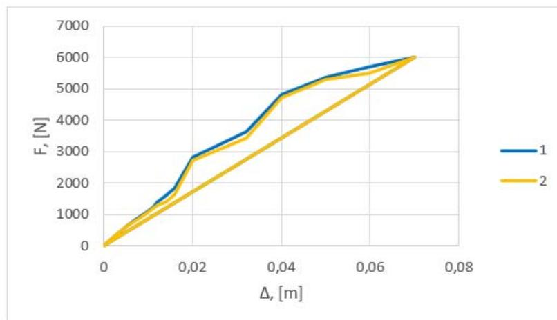
Fig.9. Modification of the deformation of a tire of size 205/55R16.
