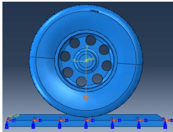
Fig.14. Application of external loads.
