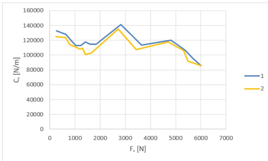
Fig.10. Modification of the elastic constant of a tire, size 205/55R16.
