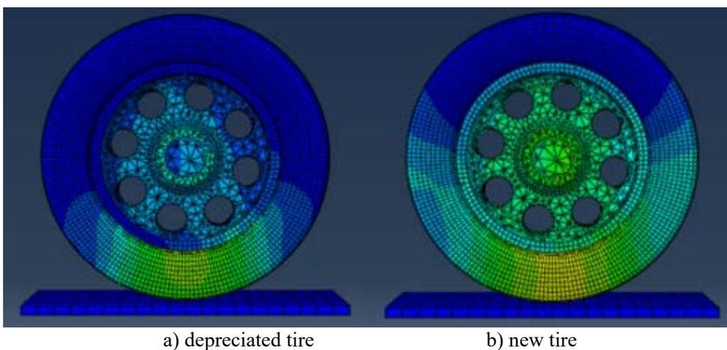
Fig.15. Deformation of a pneumatic tire.
