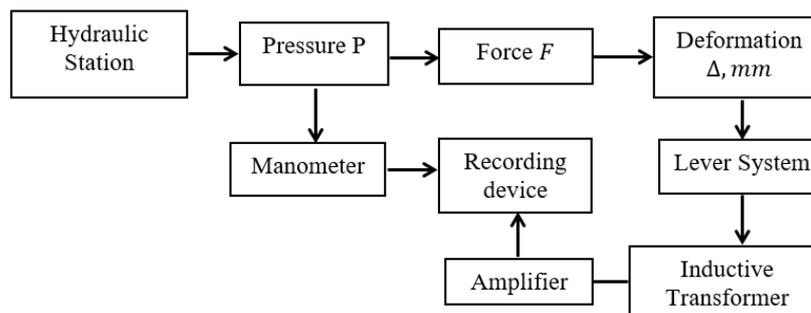
Fig.2. Block diagram for determining car tire elasticity.
