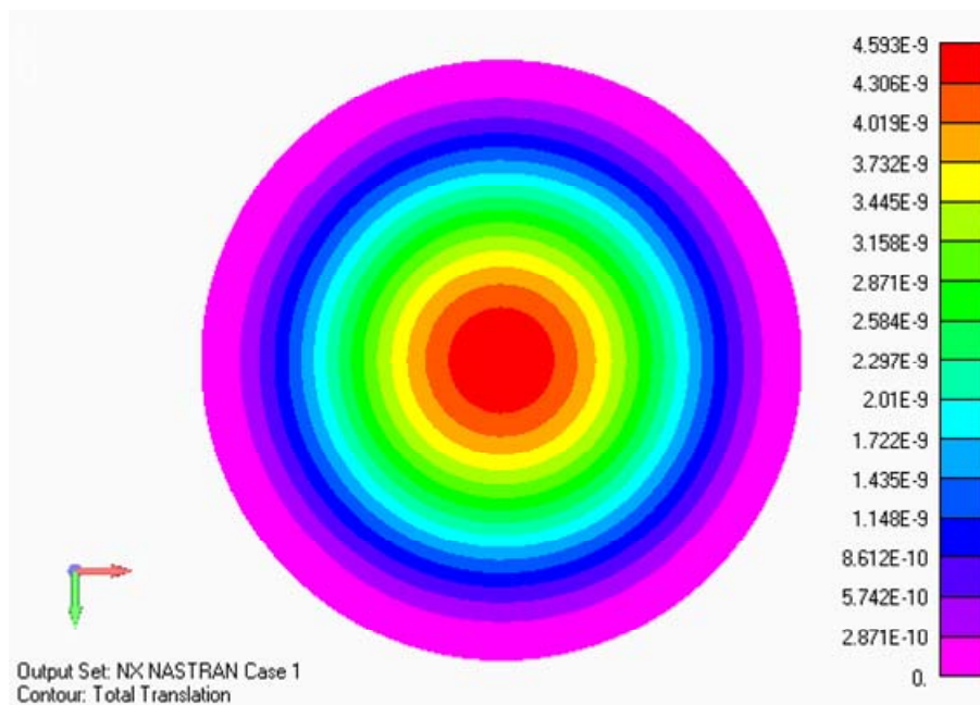
Fig.4. FEA Simulation of the <111> Silicon Diaphragm (Top View).
